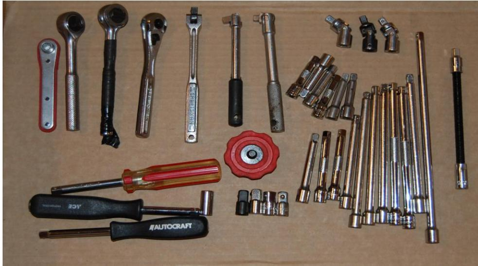
Top left: A 1/4" screwdriver bit ratchet, two cheap ratchets, a Craftsman ratchet, a Craftsman breaker bar, two cheap breaker bars.
