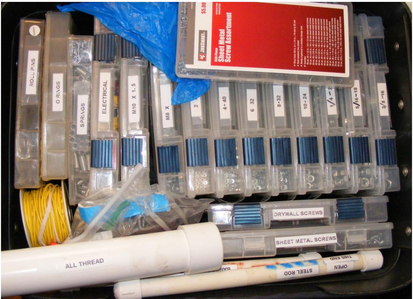
Contains: Roll pins, o-rings, springs, and a few pieces of steel rod and all-thread. Sheet metal and drywall screws also included.
