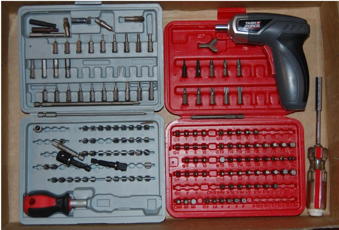
These are all the screwdriver bits I have been able to find so far. Flat, Phillips, Tri-wing, hex – SAE, metric, and tamper proof, Torx and Tamper-proof Torx, game system, and others. These are handy to have in addition to regular screwdrivers.
