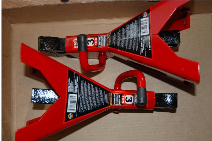
Jack stands so you're not placing your life at the mercy of a hydraulic floor jack internal seal. These should be rated for more than your vehicle weighs.
