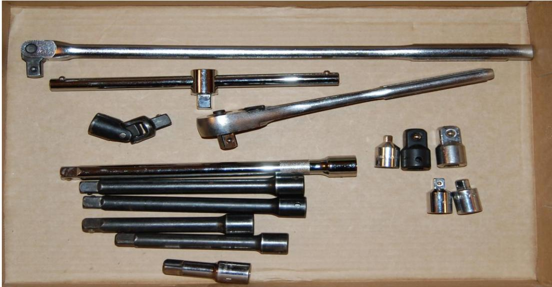
At the top is the large Craftsman breaker bar. Below that is a sliding t-handle from Tractor Supply. Then, a u-joint and Craftsman ratchet. Bottom left are extensions. To the right of those are: adapter to drive 1/4" sockets, 3/4" sockets, and 3/8" sockets.
