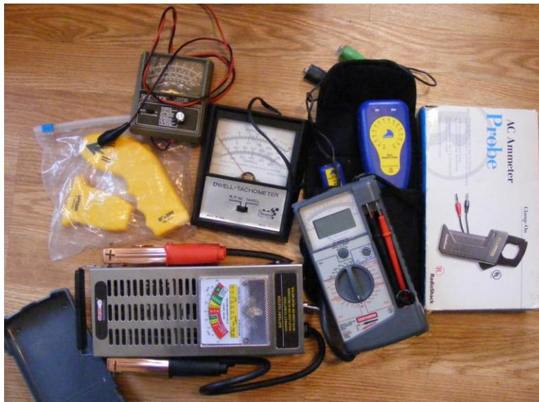
Multimeters, a battery tester, tach/dwell meter
