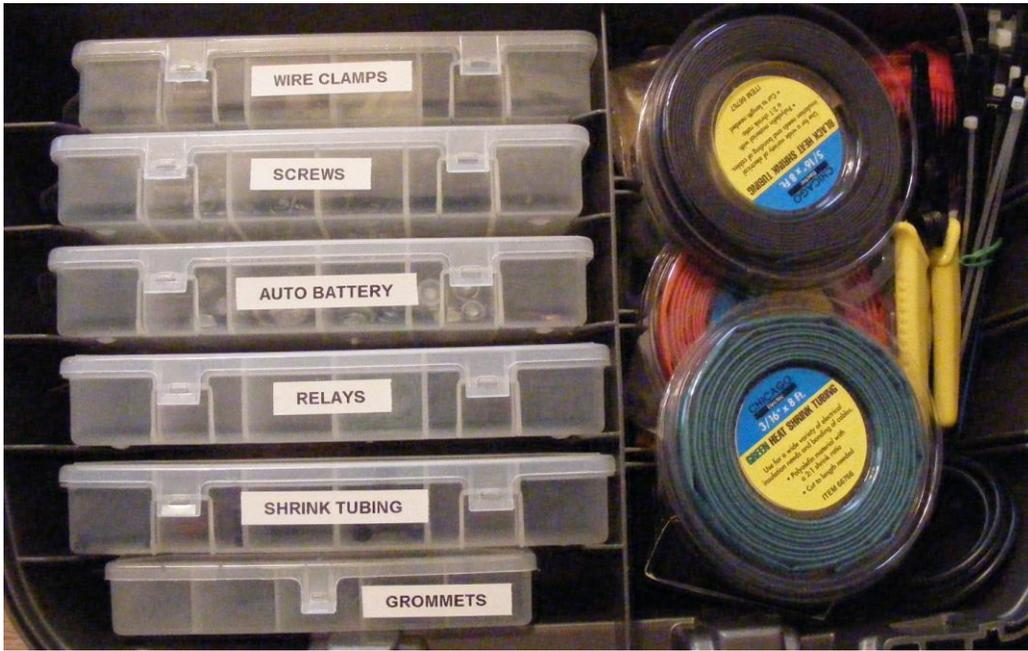
Another compartment has wire clamps, auto battery terminals, relays, grommets, shrink tubing. The compartment on the right contains spools of shrink tubing, wire strippers, and zip ties.
