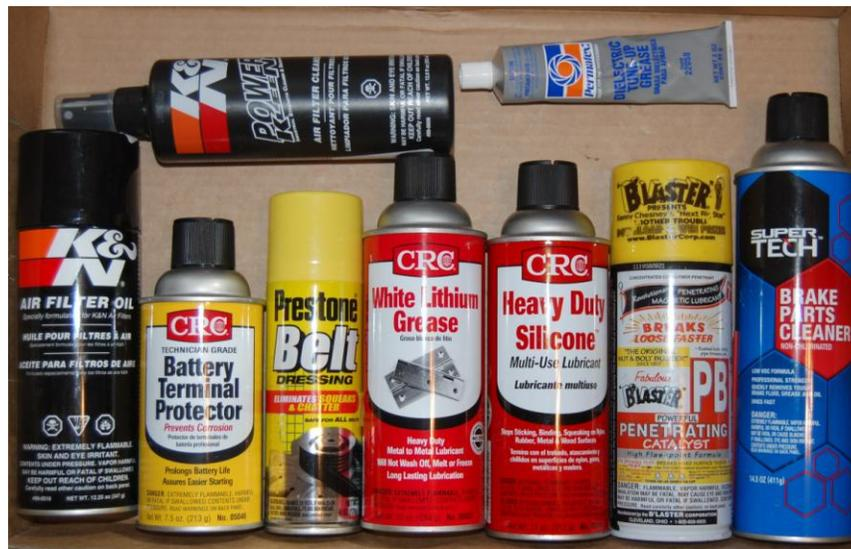
K&N air filter cleaner. Battery terminal protector. Belt dressing. White lithium grease for hinges. Silicone spray.
