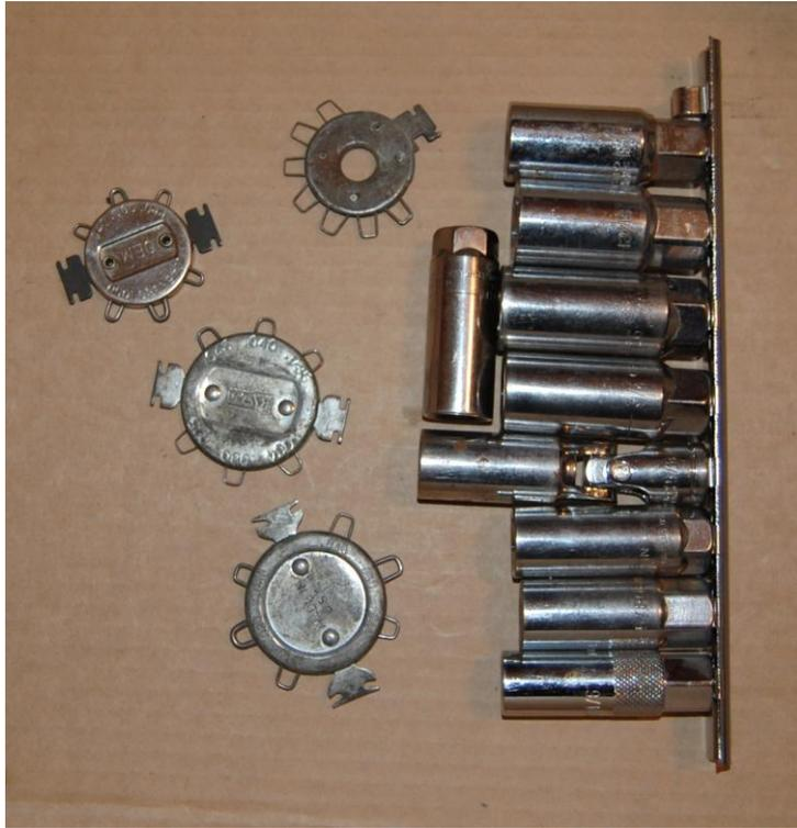
Spark plug gap tools and sockets.
