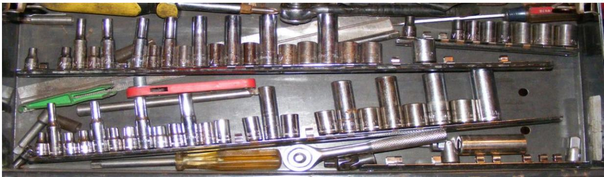
Sockets: You need both regular and deep well sockets in standard and metric. I bought a cheap set and then I have Craftsman sockets. The cheap set doesn't get used much – I haven't found something requiring a 15/32" socket yet. The Craftsman sockets get used more. You should have a name brand socket for 1/4", 5/16", 3/8", 7/16", 1/2", and possibly 11/32" in standard, and 8, 9, 10, 11, 12, and 13mm in metric.
