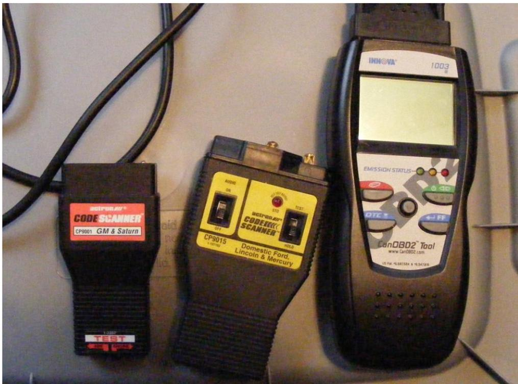
GM OBD 1 scanner, Ford OBD 1 scanner, and an OBD 2 scanner
