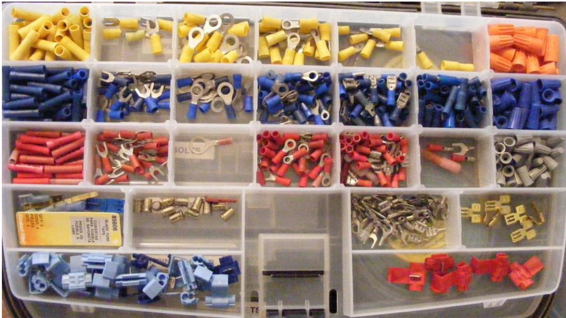
These are assorted wire terminals for different sizes of wires.
