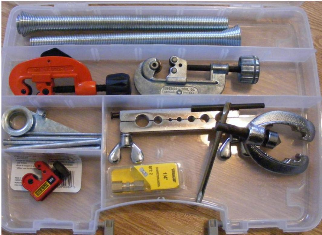
At the top are spring tubing benders – you place the tubing inside the spring so it doesn't collapse when you bend it. Below that are tubing cutters. On the left is another tubing bender and a few smaller spring tubing benders. Below that is a miniature tubing cutter. To the right of that is a single flare tool – not for use on brake lines which need double flared or compression fittings.
