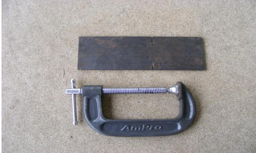
A C-Clamp and flat metal bar for pushing caliper pistons back in. Size of C-clamp varies with vehicle.
