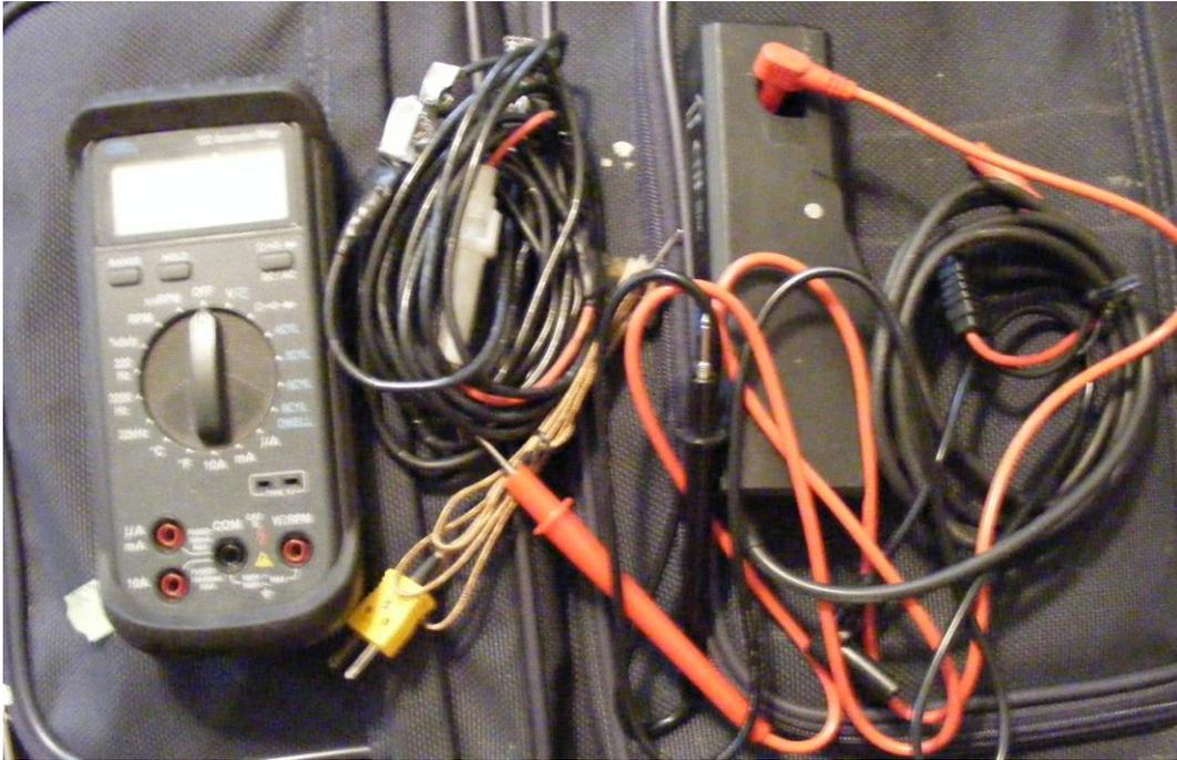
A meter with temperature and RPM leads.
