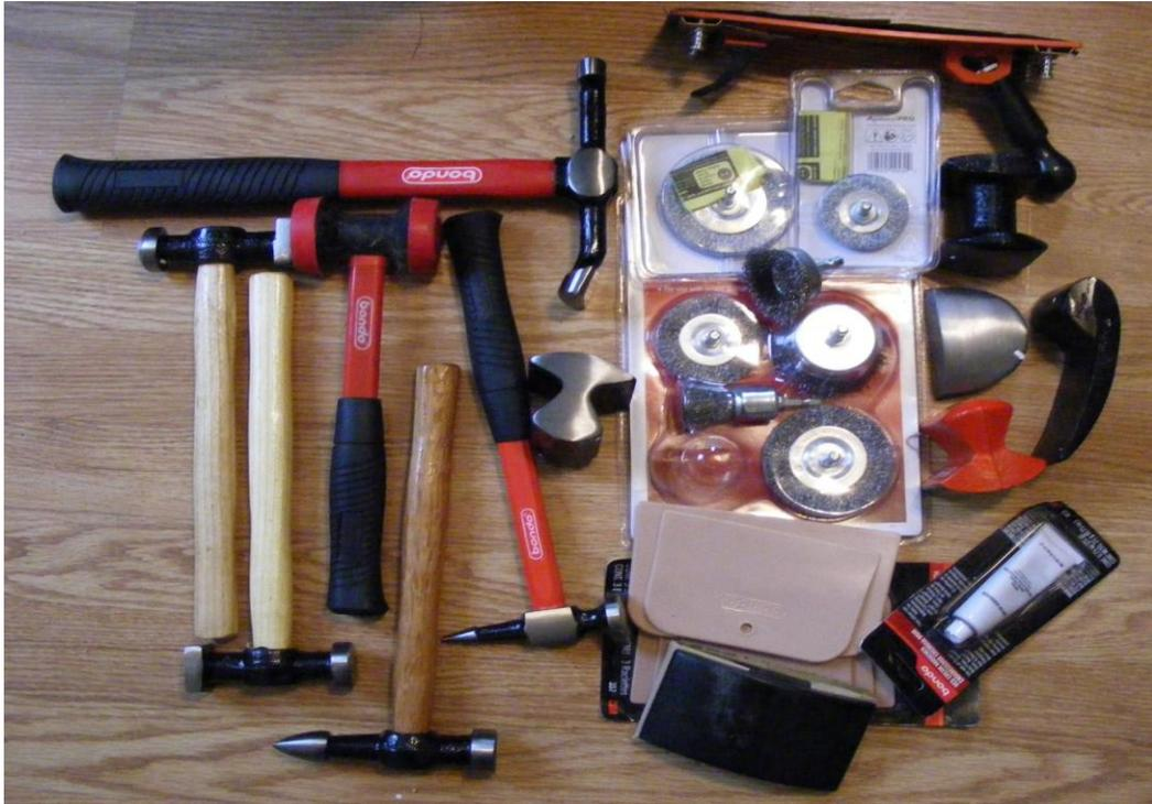
To the left are body hammers. In the middle are wire wheels for a drill, body filler spreaders, and sanding blocks. To the right are a few dollies to have something to hammer against.
